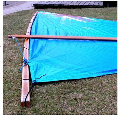
Note that the pic right shows the amount of mast bend from the correct tensioning of the snotter. The sail has been temporarily tied out at the bottom by tying to the mast base for demonstration purposes. That rope will tie to the deck saddle.
