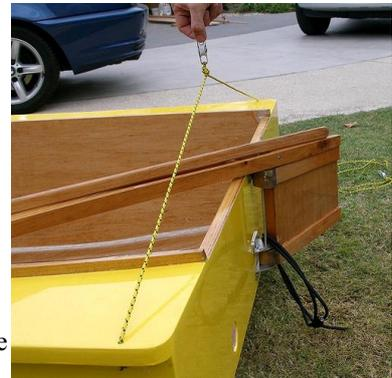
Note that our rudder fittings are homemade ones. The timber gudgeons on the rudderbox are hardwood with lots of layers of fibreglass tape (5) wrapped round the radius and running onto the faces of the rudderbox about 50mm. A trick is to put the pin through both before attaching them to the box so they will glue up aligned correctly.
