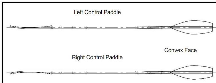
The paddle with right hand control is much more common. The right hand twists slightly at the wrist to present each blade in turn to the water. The shaft is allowed to rotate freely in the left hand.
