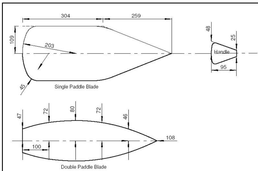
Use the supplied Blade Templates to mark the shapes on 3mm ply. There are two pieces (laminations) needed per blade.
