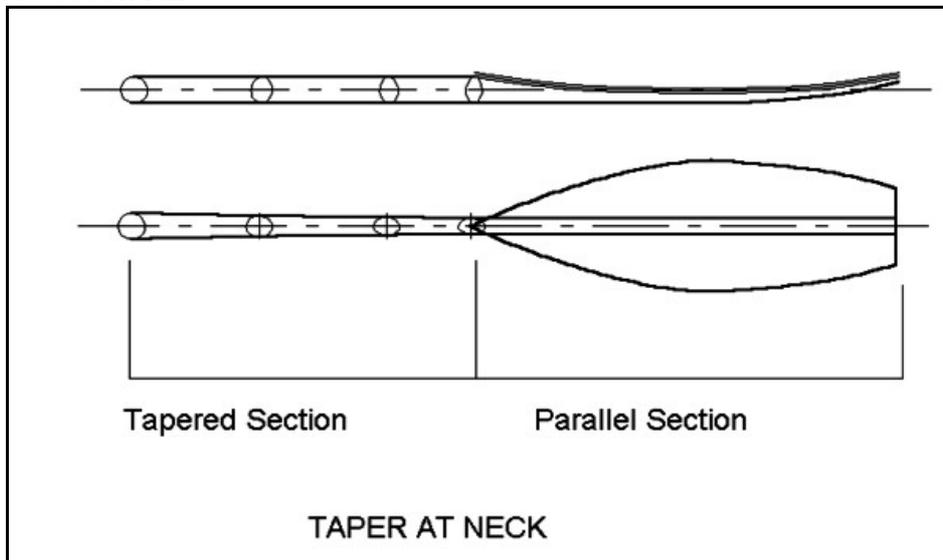
See the diagram above to see how there is a sudden change in shape at the shaft neck, where the blade will attach. The ellipses show the cross section changes at different heights – circular at the left hand side altering to an ellipse.
