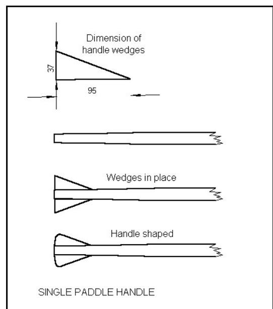
Apply glue to the handle triangles and clamp back in place.
