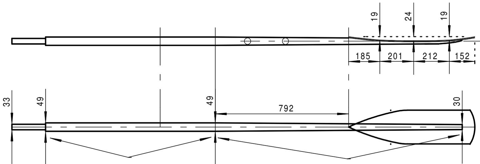
No Taper in this section 300 gsm glass between these points - 2 layers
