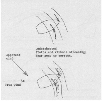
Correct (Tufts and ribbons stream, but sometimes agitated) Adjust upper main with sheet and/or vang until main leech ribbons stream or collapse at same time as jib tufts, then steer for streaming with occasional agitation.
