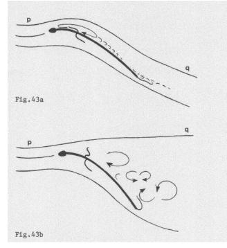
In Fig.43b the sail has been sheeted in so far that the airflow has separated from the leeward side of the sail. The leech ribbon has collapsed behind the leech. The flow line pq is now blowing straight downwind, not attempting to follow the sail's curve at all. If there is no curve there can be no suction, so the total thrust from the sail has decreased substantially. This sail is said to be stalled.
