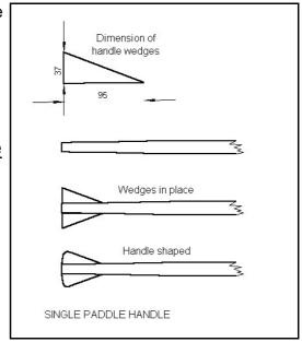
Apply glue to the handle triangles and clamp back in place.
