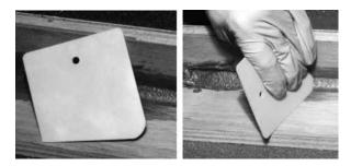
**Figure 11-22** An alternative filleting tool can be made by cutting an 808 Plastic Spreader with the desired fillet radius and the adjoining sides at 75° angle. With an adequate amount of thickened epoxy in the joint and by holding the tool at the proper angle you can make a smooth fillet in one pass. The sides of the tool will force all of the excess epoxy toward the fillet and leave a clean margin on either side.
