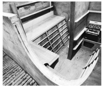
**Figure 26-7** *Rogue Wave's* galley, pilot berth, navigation area, and daggerboard case. All interior joinery was installed before the deck was built. Circular pads on the bulkhead are reinforcing gussets. Note the lift-out access ports in the cabin sole. The unfinished teak cockpit sole is visible at the lower left.
