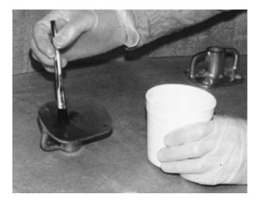
Figure 14-13 Apply epoxy to the bonding surface.
