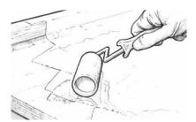
**Figure A-21** Wet out porous surfaces before applying fairing compound.
