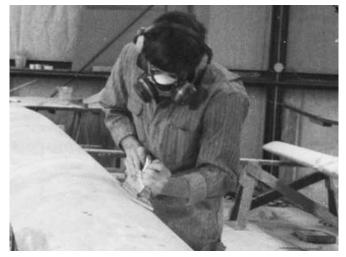
Figure 8-5 Using an air-powered file with the standard  $2^{"} \times 14^{"}$  pad.
