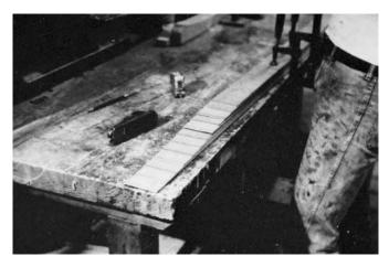
**Figure 12-11** Planing narrow plywood strips with a block plane.
