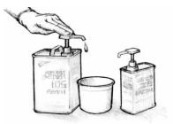
**Figure A-2** Dispense the proper proportions of resin and hardener. With Mini Pumps—pump one full stroke of resin for every one full stroke of hardener.
