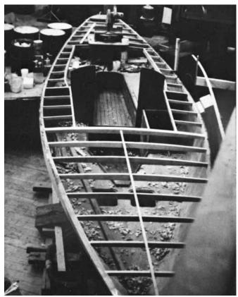
**Figure 27-31** The deck of a 26' (7.9m) Luders 16 framed-in and ready for plywood covering.
