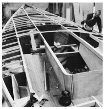
Figure 27-9 A hanging cockpit supported by longitudinal beams.
