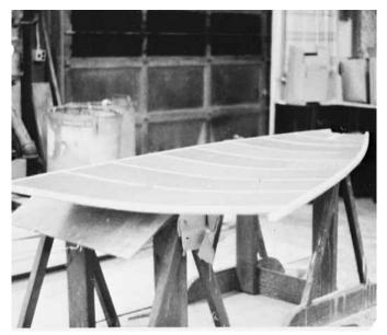
**Figure 11-16** A cockpit sole with a curved shape using core laminates. This was accomplished by laminating a curve in the frames before they were bonded together.
