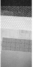
In sandwich construction, fiber reinforced resin serves as the structural skin of a part. Separating two structural skins with a core material will improve the composite's stiffness and reduce weight, much like the web of an I-beam separates the flanges. Cores can be of plywood, end-grain balsa, foam or honeycomb. Normally, the core is much lighter than the skin material. Like most materials, different cores have advantages and disadvantages.
