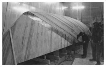
**Figure 23-9** Laminating a second layer of veneer onto a strip planked hull.
