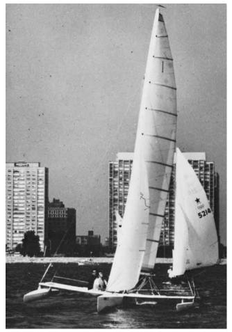
**Figure 25-1** *Victor T,* a lightweight, 25' (7.6m) C-class trimaran, was built using compounded plywood technique.
