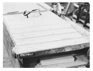
Figure 12-13 Cutting scarf bevels on stacked panels.
