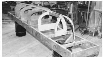
**Figure 18-1** The strongback and mold frames for a small canoe. Note that it's often a good idea to raise a small strongback off the floor to a convenient working height.
