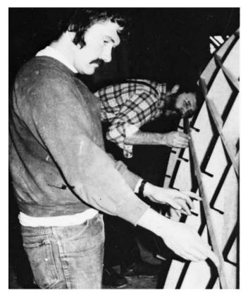
Figure 22-7 Fairing the molds on a stringer-frame set-up.
