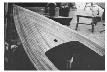
**Figure 27-34** Deck planking and final sanding are completed. Note the herringbone pattern where planks meet along the centerline. Also note that the teak begins several inches inboard from the sheer to allow for a painted cover board for an attractive effect.
