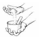
**Figure A-5** Stir in small handfuls of filler until the desired consistency is reached.
