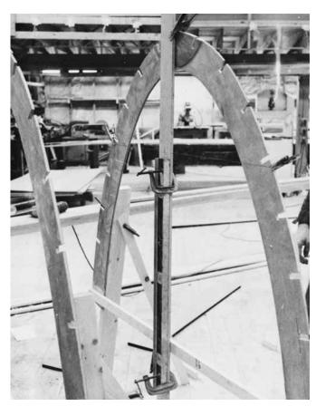
Figure 18-7 A straightedge clamped at centerline of frame.
