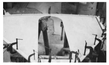
Figure 17-7 Bonding cheek pieces to a permanent bulkhead.
