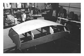
**Figure 24-11** A stitch-and-glue pram under construction. Frames will hold the shape until stitching is complete. A brace across the gunwales will hold the shape while the hull is inverted and the interior joints are filleted and taped.
