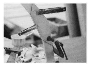
Figure 17-6 Bonding gussets to permanent frames.
