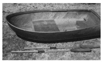
**Figure 5-3** A molded dinghy built by Peter Unger. This size and style are ideally suited to the mold method.
