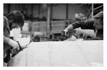
**Figure 21-7** Stapling veneer plank to a hull's stringers. Note the use of plastic strips under the staple heads to ease removal.
