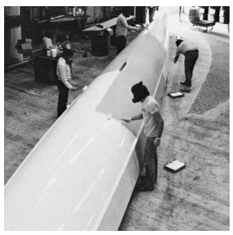
Figure 15-6 Rolling on two-part linear polyurethane paint.
