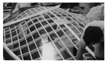
**Figure 27-11** Laminated frames and 1"  $\times$  <sup>3</sup>/<sub>4</sub>" (25mm  $\times$  18mm) stringers used as framing for a blister-type deck on a <sup>1</sup>/<sub>2</sub> ton racer. Note the plywood mast partner for a keel-stepped spar.
