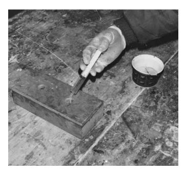
Figure 14-10 Use a syringe to fill oversized holes.
