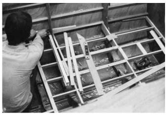
**Figure 26-18** Installing cabin sole framework in *Rogue Wave*. The structure supports the hull skin as well as the cabin sole.
