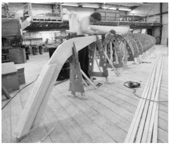
**Figure 19-2** The laminated stem for the proa *Slingshot*. The extra blocking on the side of the stem is for the slight flare in the bow. Note the set-up cable on the floor and the notch for the cable in the stem at the lower left corner of the photo.
