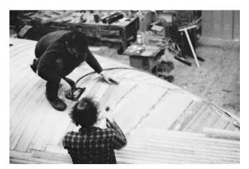
**Figure 21-21** Applying the final layer of veneer on IOR 2-ton *Golden Dazy.* Topsides of this layer were laid fore and aft, and bottom veneers laid athwartship and butted as in the photo. Note that the layer of veneer below the final layer is of much wider veneers.
