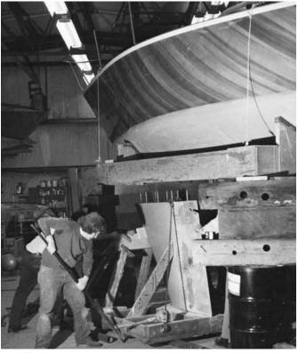
**Figure 14-24** Rolling a 10,000-pound keel into position on a handling fixture. The keel can be shifted slightly from side to side and fore and aft.
