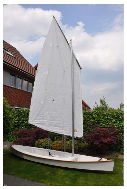
A square lashing to keep the boom near the mast is not necessary when using Dyneema in the halyard and downhaul (the boom will not really move away from the mast). Some people like to fit more sail controls like a vang or a bleater allowing one to move the downhaul back a bit on the boom creating a vanghaul (more information can be found on www.storerboatplans.com).
