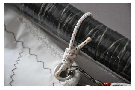
The outhaul fitted allows quick and precise adjustments to the depth in the bottom part of the sail. The maximum depth (1:7) is pre-set by having a roper stopper in the control line.
