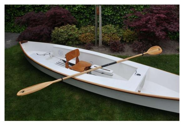
The seat you see in the photos has a back that folds away allowing for easy storage and was specially designed for the Viola 14 canoe (plans available on <u>www.duckworksbbs.com</u>). It also doubles as a comfortable seat when making camp.
