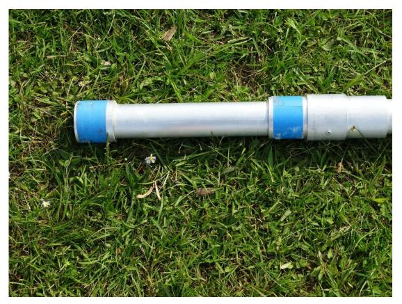
Next slide the top mast section in the bottom mast section. Wrap some electrical tape around the joint to make the mast watertight and to avoid the joint being able to pinch the fabric of the sail and to keep the deadeye in the top of the mast at a 90 degree angle to the horn cleat at the bottom of the mast.
