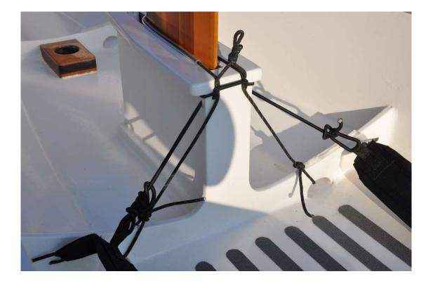
The top block of the mainsheet is attached with a carabiner to a rope loop attached with a prusik knot to the boom. Tie the aft end of the main sheet to the boat or put a figure of eight in or both (the knot prevents the boom to go out more than 90 degrees and because the sheet is also tied to the boat, you can easily find it).
