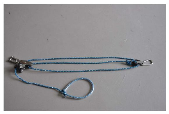
The downhaul is easily fitted in place by having a carabiner on each end. One end clips in a rope loop fitted next to the mast and the other end in the rope loop attached with a prusik knot around the boom. Rope loops on the boat (and your spars) are cheap, very strong and soft to the body.
