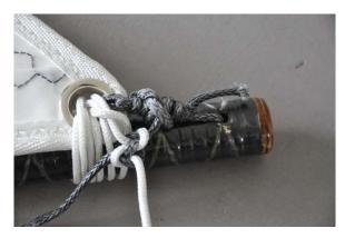
When tying on the sail, what you are a looking for is a slight crease in the sail along the length of the yard. It follows from the above that this crease should be there when the sail set, not when the sail is down since the throat being pulled down by the tension on the luff is the starting point. The crease disappears when the wind fills the sail.
