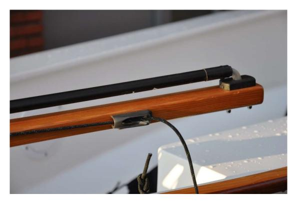
In the photos the downhaul consists of a 3mm rope with Dyneema core pre-lead line and a regular polyester 4mm control line that stretches. Due to the stretch in the downhaul control line it is easier to tension the downhaul and to get it out of the cleat again.
