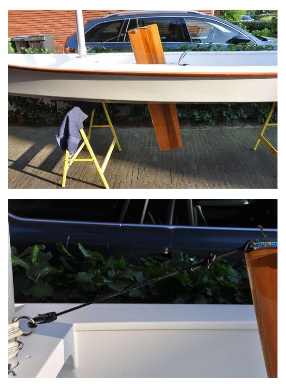
The plastic hook allows for quick (de)rigging.
