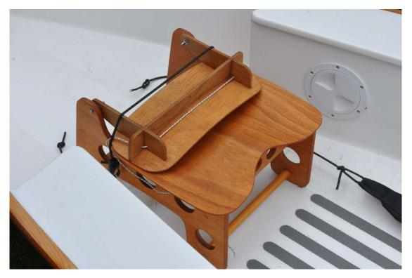
Useful for paddle sailing is a thwart spanning the width of the boat (essentially a simple plank) held in place with a piece of bungee cord. The edges on the underside of the one in the photos have bevelled as to shed some weight and to give it a lighter appearance. 4 wooden dowels glued and screwed in place keep the seat in the right position and prevent it from sliding aft. These dowels have been spaced such that the seat rests on the top of the
