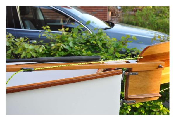
A 900mm long tiller extension is suggested mounted right at the front of the tiller.
