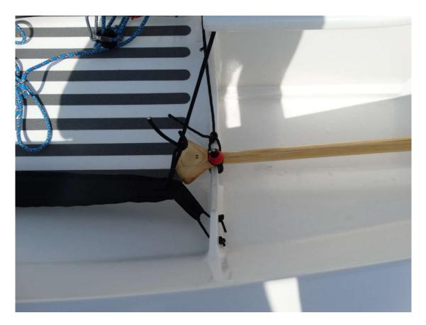
A paddle/paddles is/are easily secured to the boat using 2 elastic loops and the limber holes in the front frame and the mid frame of the boat. Again rope stoppers are used on the elastic loops that thus quickly fasten around the limber holes and the paddle. To avoid losing them when not fastened up, the elastic loops can be kept in place on the limber holes using some Velcro.
