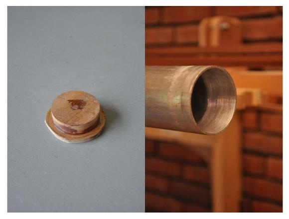
Next glue the plug that you just created in place. When the glue has hardened, trim the outside of the round that overlaps the tube's sidewalls to size.
