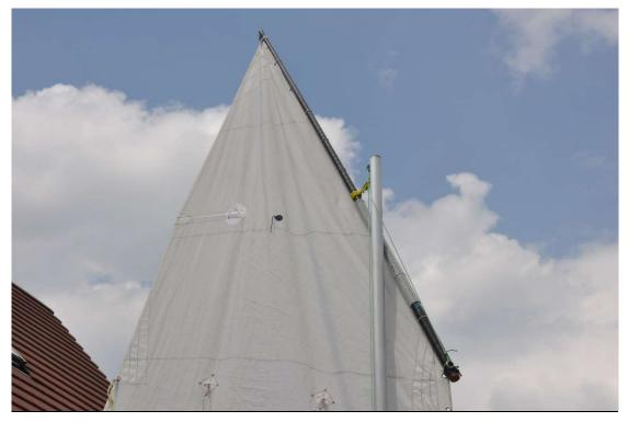
In the photo's you see a stainless steel ring tied to the front of the halyard with some Dyneema rope - the stainless steel ring is easier to work with in challenging (wet and/or cold) conditions when having to attach the halyard to the yard.
