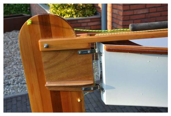
Do not overtighten the nuts on the bolt, just tighten them up by hand. If using 2 nuts on each end, one can tighten these against each other using spanners and this will avoid them coming loose. Use cap nuts on the outside to avoid having any sharp bits.
