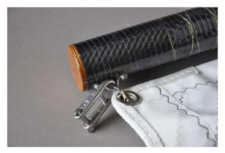
The clew of the sail is attached as shown below in the section dealing with the outhaul. A rope loop (in this case 4mm Dyneema) keeps the clew near the clew.
