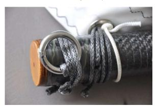
It takes a bit of trial and error, but quickly you will find the correct peak tension that will not result in the tension on the luff progressing in the head of the sail, but giving the right tension on the head getting rid of wrinkles and such. If there is too much tension on the head of the
