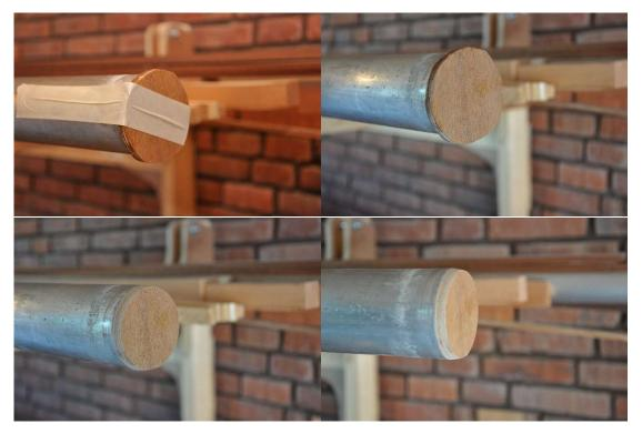
Lastly apply varnish or paint (epoxy optional) to protect the plywood.
