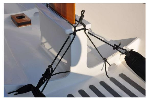
A piece of plastic tube reduces friction when pulling the foil up or pushing it down.
