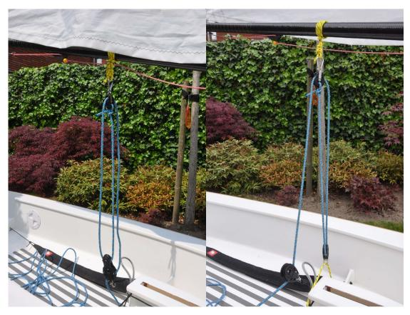
For cruising a block with camcleat may come in handy if having to paddle sail. If using a block with camcleat, make sure that the camcleat points up so you cannot accidently cleat your mainsheet and it is easy to pull the sheet out of the cleat if so required.
