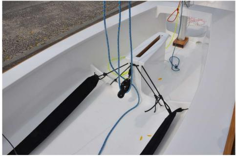
The front end of the hiking straps are lifted of the sole by 6mm elastic that is fed through 2 holes in the mid frame next to the dagger board case. The elastic also keeps in place the top end of the rope bridle that is knotted to the limber holes in the mid frame. All soft attachment points, cheap and easy.
