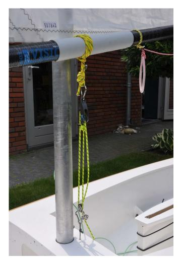
Alternatively, you could use a system using a fiddle block with a camcleat.
