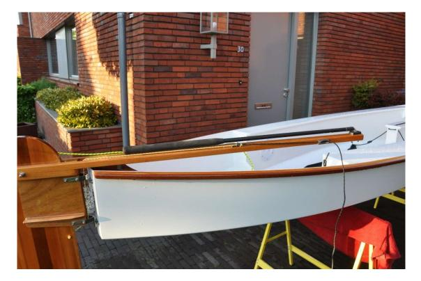
The rudder uphaul is a very simple affair on the Viola 14 canoe. A hole is drilled in the rudder head aft of the centreline of the foil and a rope is attached to this hole by a simple knot on the opposite side of the where the clam cleat for the uphaul is located (please refer to the first photo on the rudder and its controls above for the exact location of the hole in the rudder head). Obviously the same comments apply in respect of making an epoxy bushing for the uphaul attachment hole.
