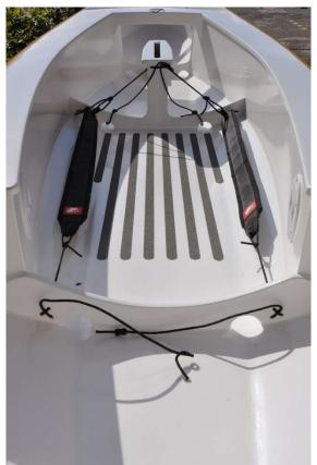
The front end of the hiking straps are attached to a rope lope fed through 2 holes drilled in the mid frame. Further down there is another more detailed photo.
