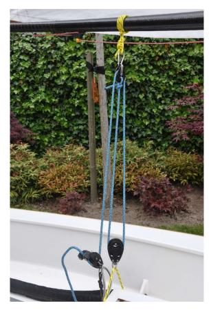
All of these systems use only 3 blocks allowing quick adjustments since you do not have to pay out/take in much sheet, which is in line with this type of boat that requires active sailing. Use a ratchet block to keep the loads manageable.
