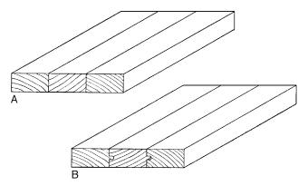
Figure 9–8. Edge-grain joints: A, plain; B, tongue-and-groove.
