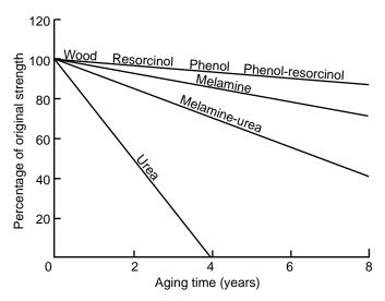
Figure 9–12. Relative rates of deterioration of bond strength of small specimens exposed directly to weather.
